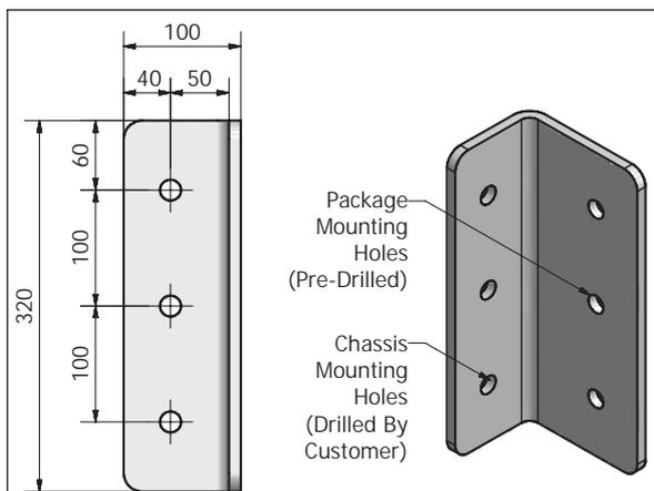
Figure 4f - Recommended Vehicle Chassis Mounting Bracket Hole Positions.
