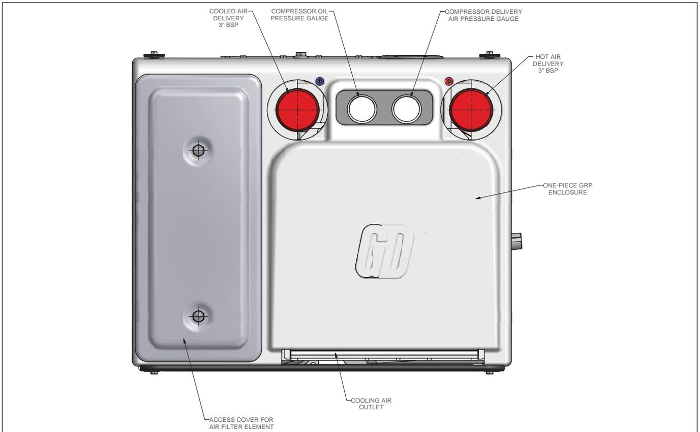
Figure 2a - Components Front View Clockwise (Right Hand) Rotation
