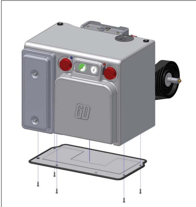
Figure 5e - Underside Cover Removal
