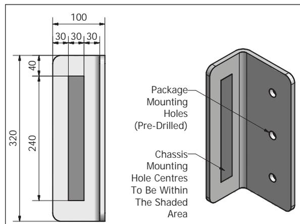
Figure 4g - Permissible Vehicle Chassis Mounting Bracket Hole Positions.
