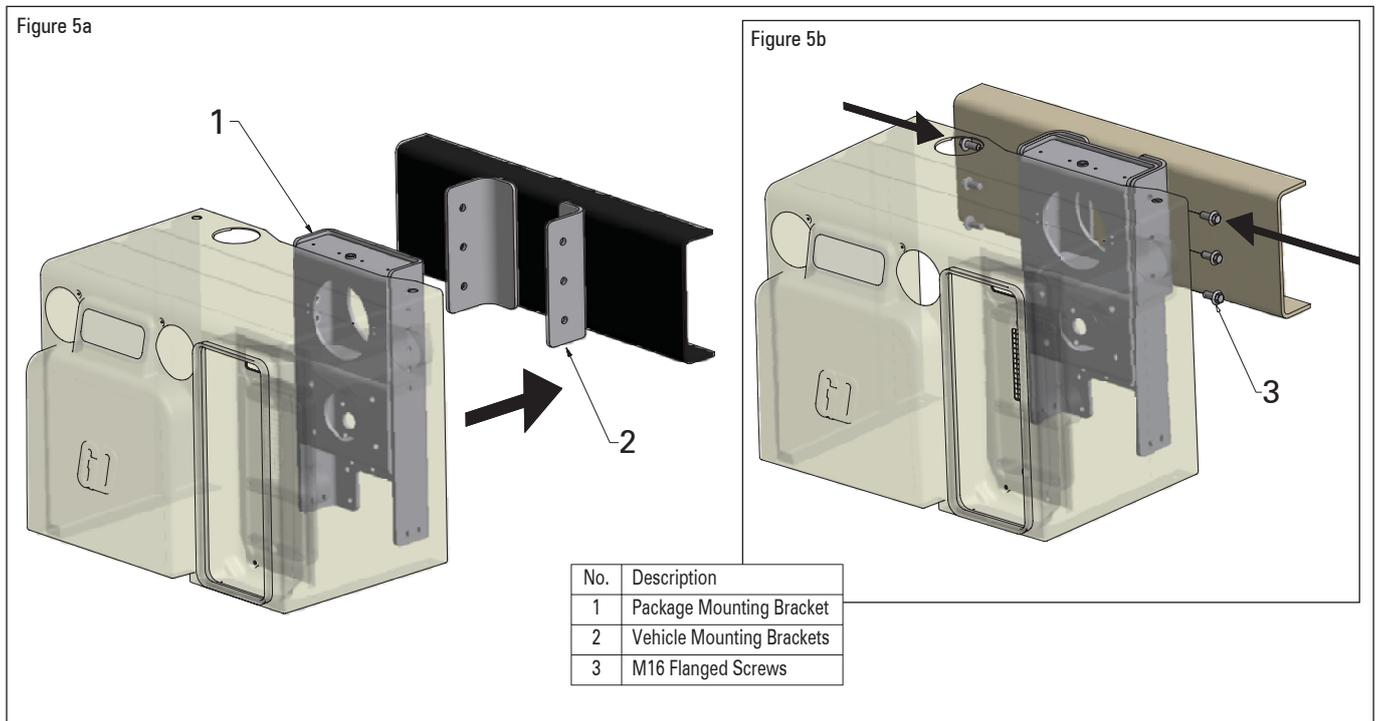
Figure 5 - Installation of Bulkline 650/1000 LNC Package to the Vehicle Mounting Bracket/Chassis
