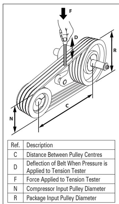
Figure 12. Belt Tension Testing
