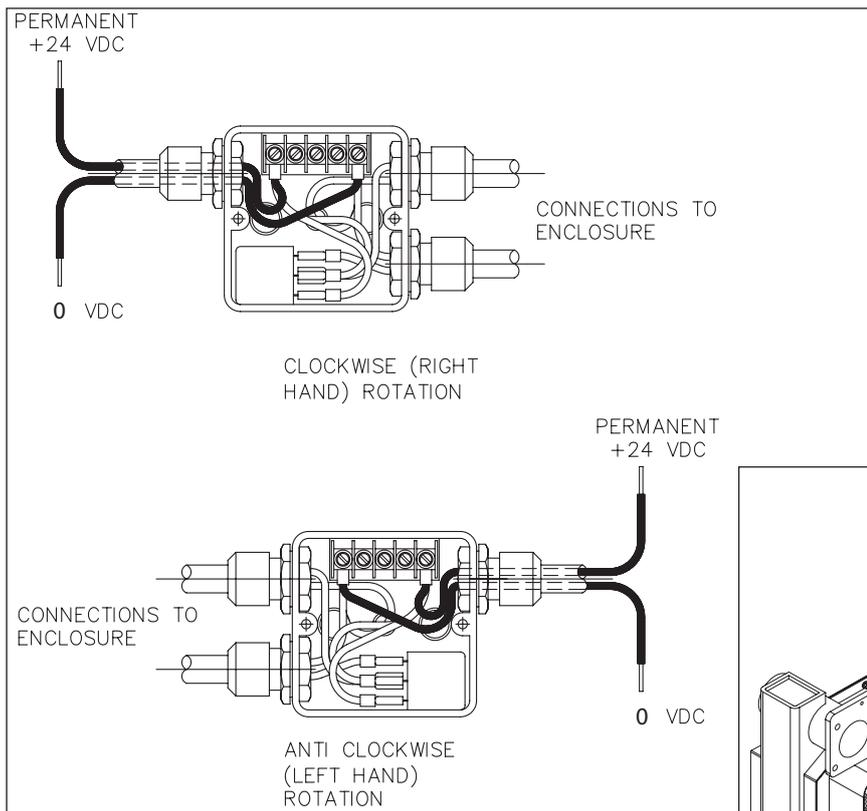
Figure 11c. Junction Box Connection Diagram
