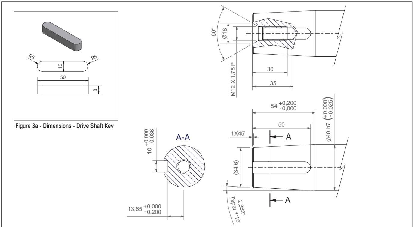
Figure 3a - Dimensions - Drive Shaft Key
