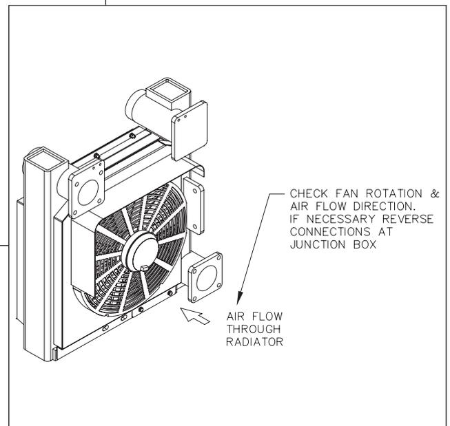
Figure 11d. Air Flow Direction
