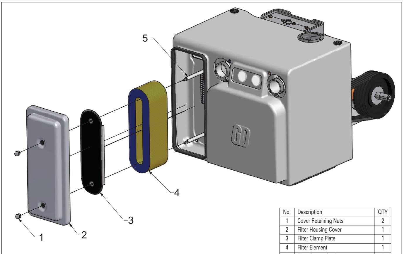
Figure 13b. Replacing the filter element
