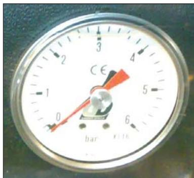
Figure 8 - Discharge Air Pressure Gauge Display
