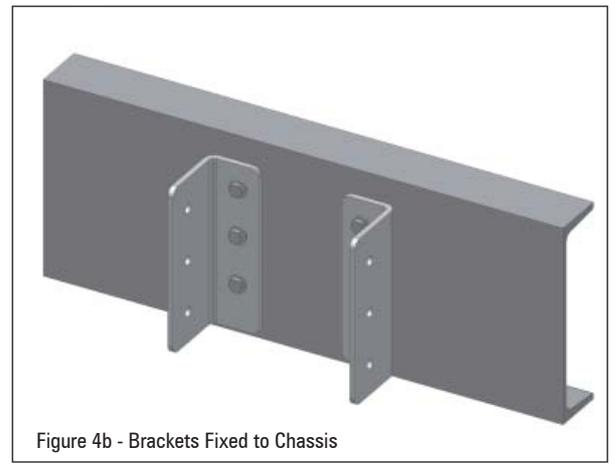
Figure 4b - Brackets Fixed to Chassis
