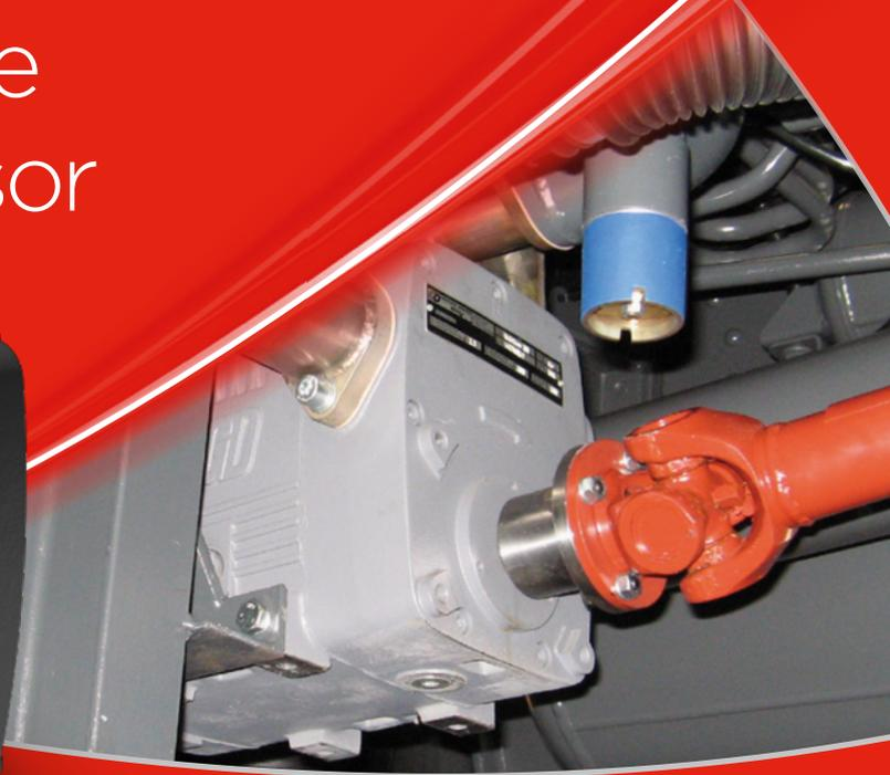
The SC200 screw compressor is specifically designed for the contaminant free discharge of bulk liquid products, such as liquid foodstuff, solvents, acids, alkalis, hot bitumen and other chemicals from general purpose tankers. The compressor has no wearing parts in the main compression cavity which provides low operating and maintenance costs.
