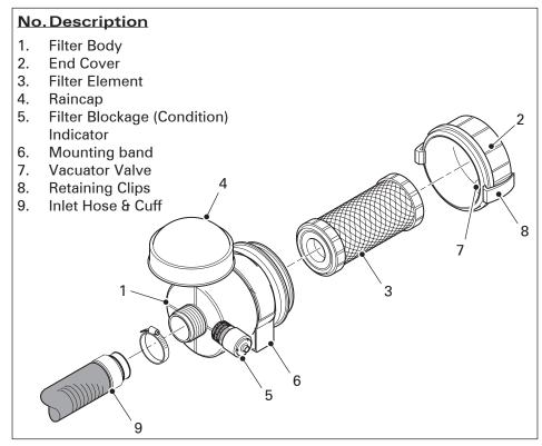
Figure 9. Replacing Air Filter
