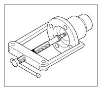
Figure 6. Drive Flange Removal
