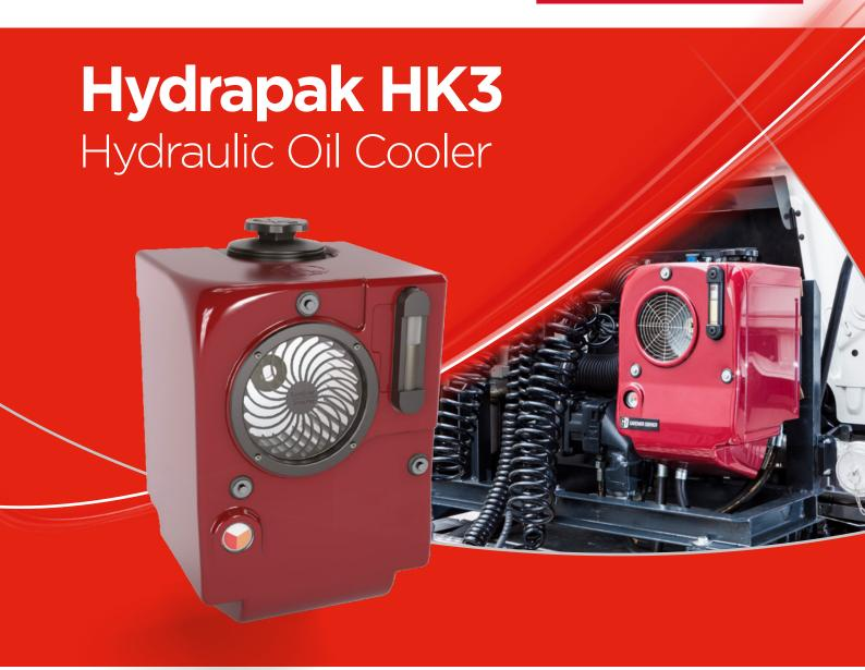
The Hydrapak HK3 Oil Cooler is an efficient, lightweight, compact oil cooler combining the oil reservoir, oil filter, control and safety equipment required in a hydraulic system within one assembly.
